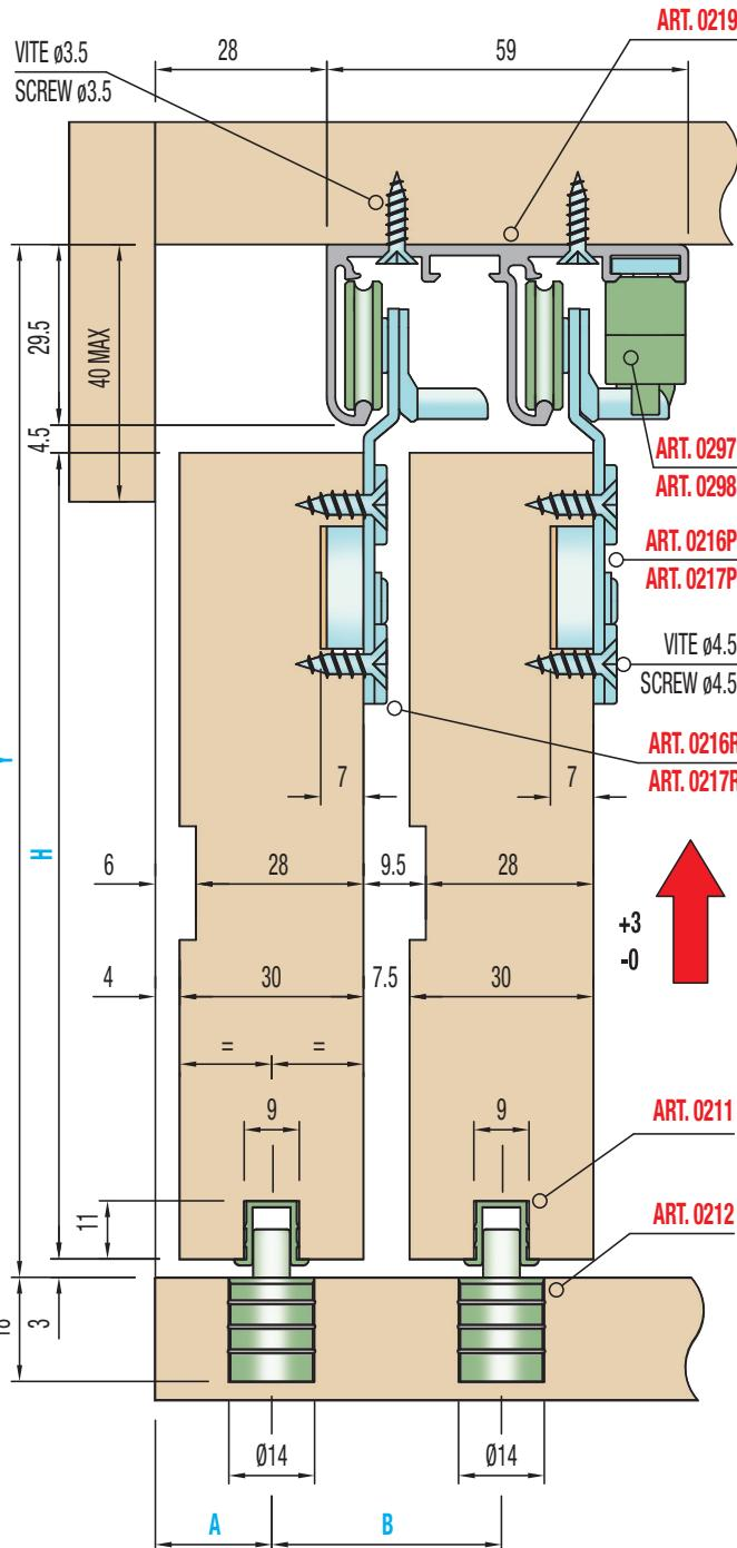
**Anta interna / Inner door****KIT 0216P-0297 - MAX 25 KG**
