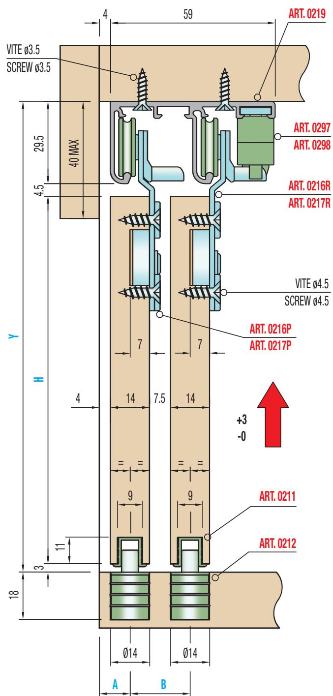
**Anta interna / Inner door****KIT 0216R-0297 - MAX 25 KG**
