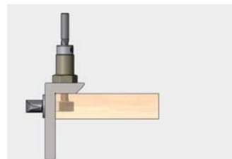
2. Drill hole 6 mm
