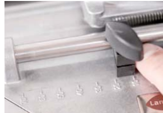
2. Adjust cutting depth
