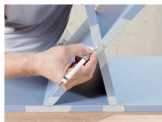
2. Copy the center to the second workpiece
