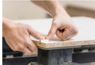
2. Insert one-piece connector
