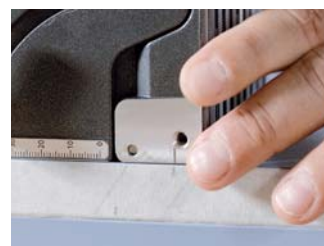
3. Align the Zeta P2 with the marking
