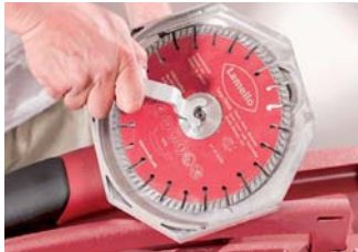
1. Use diamond disc or saw blade
