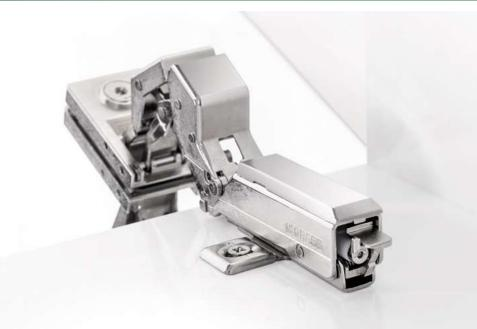
Tiomos Mirro is secured on the glass side of the door with an eccentric cam on a Zamak adapter. It is not necessary to drill a hole in the glass. This fastening method ensures firm attachment and has a light, floating look.
